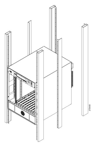
You can install your Cisco RFGW-10 chassis in a two-post rack (see Two-Post Rack Installation Mid-Mounted, page 15) or a four-post rack.
